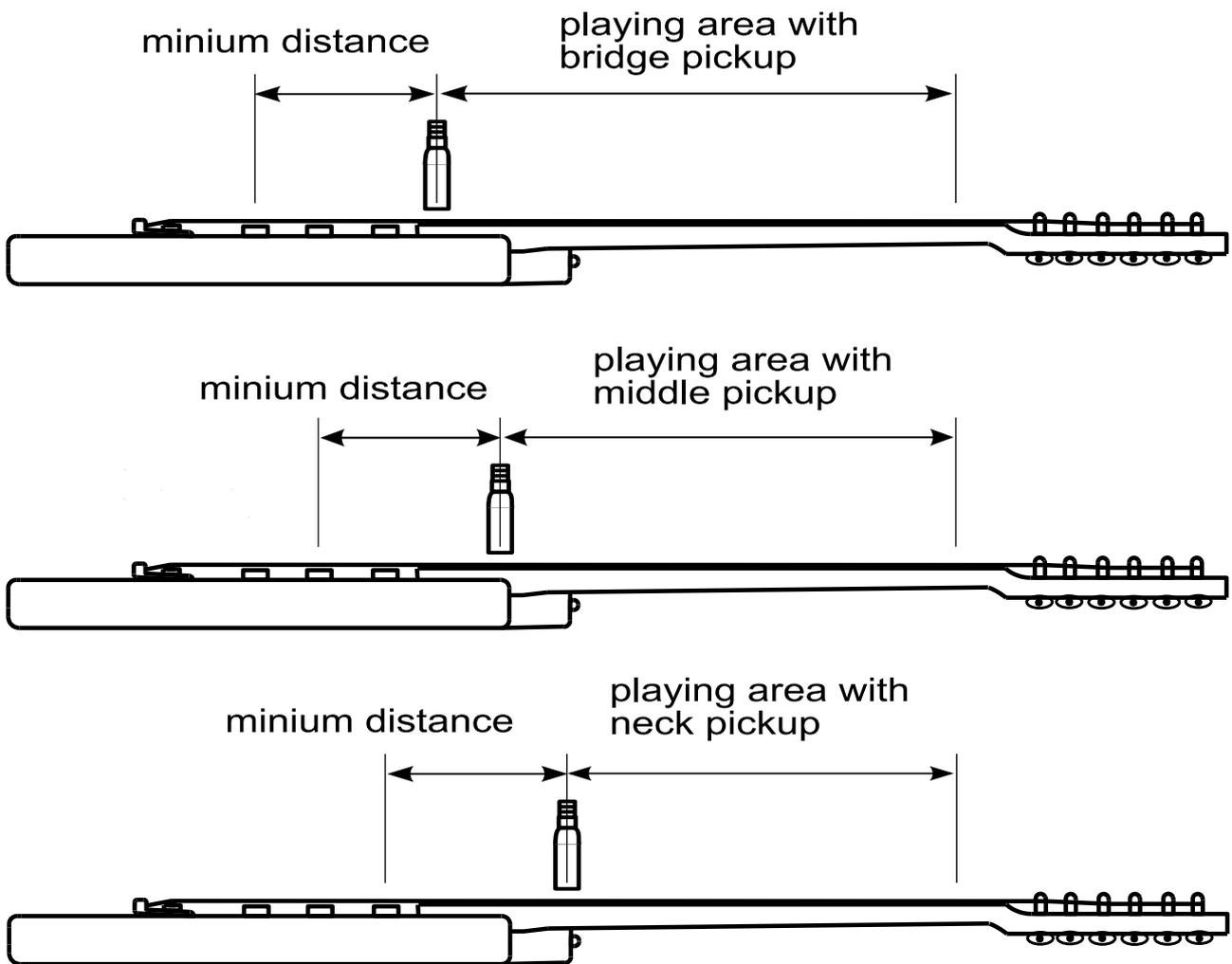
The sensitivity not only depends on the Resonator power but also on the pickup. In general humbucker show less sensitive than single coils. With some practice you play closer by the strings which enables you to reduce the Resonator power. Then, you can also play with the neck pickup (or middle pickup). You should absolutely work it out, because these feedbacks are sounding very rich and amazing !
